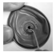
If the cuts are not completely through the center of the diaphragm nipple, do not use the diaphragm. MSA will replace diaphragms that do not have three distinct slits in the diaphragm nipple.
